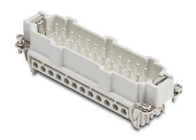
ZIPport male insert, connector housing size 24B, 24-pole, screw terminals, accepts wire size 20-14 AWG, 16 amp, 600 VAC/VDC, poles numbered 1 to 24. For use with ZIPport multi-wire housings.
