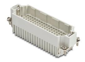
ZIPport male insert, connector housing size 24B, 108-pole, crimped contact, 10 amp, 600 VAC/VDC, poles numbered 1 to 108. For use with ZIPport multi-wire housings. Requires 10 amp male contacts ZP-MC-CC-M10A-xxx.
