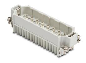
ZIPport male insert, connector housing size 24B, 64-pole, crimped contact, 10 amp, 600 VAC/VDC, poles numbered A to D/1 to 16. For use with ZIPport multi-wire housings. Requires 10 amp male contacts ZP-MC-CC-M10A-xxx.
