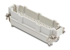
ZIPport male insert, connector housing size 24B, 24-pole, crimped contact, 16 amp, 600 VAC/VDC, poles numbered 1 to 24. For use with ZIPport multi-wire housings. Requires 16 amp male contacts ZP-MC-CC-M16A-xxx.
