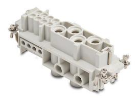
ZIPport female insert, connector housing size 24B, 12-pole, screw terminals, accepts wire size 6-16 AWG, 20-14 AWG, 80 amp (4-pole), 16 amp (8-pole), 600 VAC/VDC, poles numbered 1 to 4 and 1 to 8. For use with ZIPport multi-wire housings.
