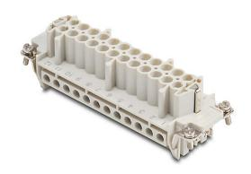
ZIPport female insert, connector housing size 24B, 24-pole, screw terminals, accepts wire size 20 - 14 AWG, 16 amp, 600 VAC/VDC, poles numbered 1 to 24. For use with ZIPport multi-wire housings.
