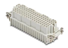
ZIPport female insert, connector housing size 24B, 108-pole, crimped contact, 10 amp, 600 VAC/VDC, poles numbered 1 to 108. For use with ZIPport multi-wire housings. Requires 10 amp female contacts ZP-MC-CC-F10A-xxx.
