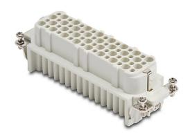
ZIPport female insert, connector housing size 24B, 64-pole, crimped contact, 10 amp, 600 VAC/VDC, poles numbered A to D/1 to 16. For use with ZIPport multi-wire housings. Requires 10 amp female contacts ZP-MC-CC-F10A-xxx.
