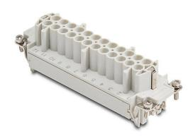
ZIPport female insert, connector housing size 24B, 24-pole, crimped contact, 16 amp, 600 VAC/VDC, poles numbered 1 to 24. For use with ZIPport multi-wire housings. Requires 16 amp female contacts ZP-MC-CC-F16A-xxx.
