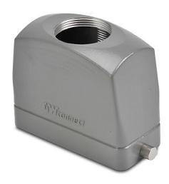
ZIPport hood housing, 2-peg, top entry, connector housing size 16B, (1) Pg 29 threaded hole, high construction, heavy-duty die cast aluminum. For use with ZIPport size 16B single lever connector housings.
