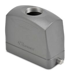
ZIPport hood housing, 2-peg, top entry, connector housing size 16B, (1) Pg 21 threaded hole, high construction, heavy-duty die cast aluminum. For use with ZIPport size 16B single lever connector housings.
