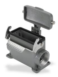
ZIPport surface mount housing, single lever, standard, connector housing size 16B, (2) Pg 29 threaded holes, high construction, heavy-duty die cast aluminum. For use with ZIPport size 16B 2-peg connector housings.
