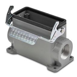
ZIPport surface mount housing, single lever, connector housing size 16B, (2) Pg 21 threaded holes, high construction, heavy-duty die cast aluminum. For use with ZIPport size 16B 2-peg connector housings.
