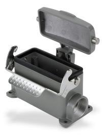
ZIPport surface mount housing, single lever, standard, connector housing size 16B, (2) Pg 21 threaded holes, heavy-duty die cast aluminum. For use with ZIPport size 16B 2-peg connector housings.
