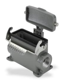
ZIPport surface mount housing, single lever, standard, connector housing size 16B, (2) Pg 21 threaded holes, high construction, heavy-duty die cast aluminum. For use with ZIPport size 16B 2-peg connector housings.
