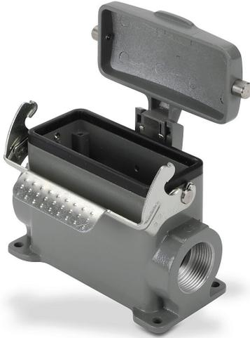
ZIPport surface mount housing, single lever, standard, connector housing size 16B, (2) Pg 21 threaded holes, high construction, heavy-duty die cast aluminum. For use with ZIPport size 16B 2-peg connector housings.
