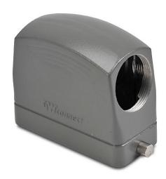
ZIPport hood housing, 2-peg, side entry, connector housing size 16B, (1) Pg 29 threaded hole, high construction, heavy-duty die cast aluminum. For use with ZIPport size 16B single lever connector housings.
