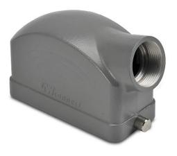
ZIPport hood housing, 2-peg, side entry, connector housing size 16B, (1) Pg 21 threaded hole, heavy-duty die cast aluminum. For use with ZIPport size 16B single lever connector housings.
