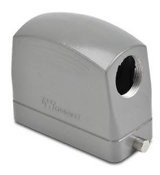
ZIPport hood housing, 2-peg, side entry, connector housing size 16B, (1) Pg 21 threaded hole, high construction, heavy-duty die cast aluminum. For use with ZIPport size 16B single lever connector housings.
