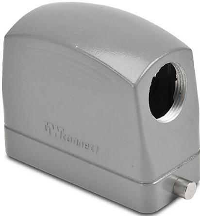
ZIPport hood housing, 2-peg, side entry, connector housing size 16B, (1) Pg 21 threaded hole, high construction, heavy-duty die cast aluminum. For use with ZIPport size 16B single lever connector housings.
