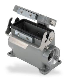
ZIPport surface mount housing, single lever, automatic closing, connector housing size 16B, (2) Pg 29 threaded holes, high construction, heavy-duty die cast aluminum. For use with ZIPport size 16B 2-peg connector housings.
