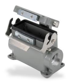
ZIPport surface mount housing, single lever, automatic closing, connector housing size 16B, (2) Pg 21 threaded holes, high construction, heavy-duty die cast aluminum. For use with ZIPport size 16B 2-peg connector housings.
