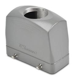
ZIPport hood housing, 4-peg, top entry, connector housing size 16B, (1) Pg 29 threaded hole, high construction, heavy-duty die cast aluminum. For use with ZIPport size 16B double lever connector housings.
