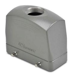
ZIPport hood housing, 4-peg, top entry, connector housing size 16B, (1) Pg 21 threaded hole, high construction, heavy-duty die cast aluminum. For use with ZIPport size 16B double lever connector housings.
