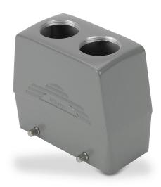
ZIPport hood housing, 4-peg, top entry, connector housing size 16B, (2) Pg 21 threaded holes, high construction, heavy-duty die cast aluminum. For use with ZIPport size 16B double lever connector housings.
