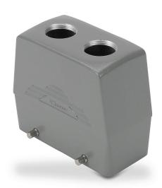
ZIPport hood housing, 4-peg, top entry, connector housing size 16B, (2) Pg 16 threaded holes, high construction, heavy-duty die cast aluminum. For use with ZIPport size 16B double lever connector housings.
