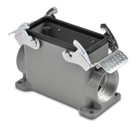
ZIPport surface mount housing, double lever, connector housing size 16B, (2) Pg 29 threaded holes, high construction, heavy-duty die cast aluminum. For use with ZIPport size 16B 4-peg connector housings.
