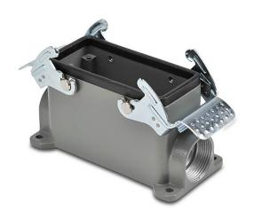
ZIPport surface mount housing, double lever, connector housing size 16B, (2) Pg 21 threaded holes, heavy-duty die cast aluminum. For use with ZIPport size 16B 4-peg connector housings.
