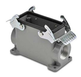
ZIPport surface mount housing, double lever, connector housing size 16B, (2) Pg 21 threaded holes, high construction, heavy-duty die cast aluminum. For use with ZIPport size 16B 4-peg connector housings.
