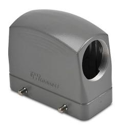
ZIPport hood housing, 4-peg, side entry, connector housing size 16B, (1) Pg 29 threaded hole, high construction, heavy-duty die cast aluminum. For use with ZIPport size 16B double lever connector housings.
