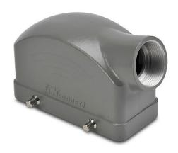
ZIPport hood housing, 4-peg, side entry, connector housing size 16B, (1) Pg 21 threaded hole, heavy-duty die cast aluminum. For use with ZIPport size 16B double lever connector housings.
