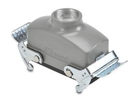
ZIPport coupler housing, double lever, connector housing size 16B, (1) Pg 21 threaded hole, heavy-duty die cast aluminum. For use with ZIPport size 16B 4-peg connector housings.
