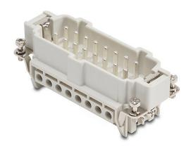
ZIPport male insert, connector housing size 16B, 16-pole, screw terminals, accepts wire size 20-12 AWG, 16 amp, 600 VAC/VDC, poles numbered 1 to 16. For use with ZIPport multi-wire housings.
