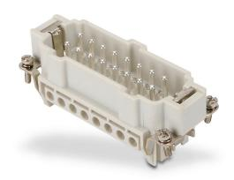
ZIPport male insert, connector housing size 16B, 16-pole, screw terminals, accepts wire size 20-14 AWG, 16 amp, 600 VAC/VDC, poles numbered 17 to 32. For use with ZIPport multi-wire housings.
