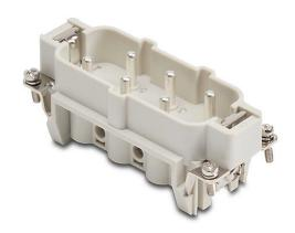
ZIPport male insert, connector housing size 16B, 6-pole, screw terminals, accepts wire size 20 - 10 AWG, 35 amp, 600 VAC/VDC, poles numbered 1 to 6. For use with ZIPport multi-wire housings.
