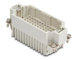
ZIPport male insert, connector housing size 16B, 72-pole, crimped contact, 10 amp, 600 VAC/VDC, poles numbered 1 to 72. For use with ZIPport multi-wire housings. Requires 10 amp male contacts ZP-MC-CC-M10A-xxx.
