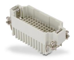
ZIPport male insert, connector housing size 16B, 72-pole, crimped contact, 10 amp, 600 VAC/VDC, poles numbered 73 to 144. For use with ZIPport multi-wire housings. Requires 10 amp male contacts ZP-MC-CC-M10A-xxx.
