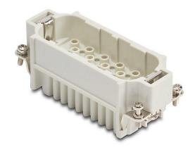
ZIPport male insert, connector housing size 16B, 40-pole, crimped contact, 10 amp, 600 VAC/VDC, poles numbered 1 to 40. For use with ZIPport multi-wire housings. Requires 10 amp male contacts ZP-MC-CC-M10A-xxx.
