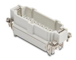
ZIPport male insert, connector housing size 16B, 16-pole, crimped contact, 16 amp, 600 VAC/VDC, poles numbered 1 to 16. For use with ZIPport multi-wire housings. Requires 16 amp male contacts ZP-MC-CC-M16A-xxx.
