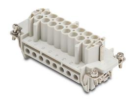
ZIPport female insert, connector housing size 16B, 16-pole, screw terminals, accepts wire size 20-12 AWG, 16 amp, 600 VAC/VDC, poles numbered 1 to 16. For use with ZIPport multi-wire housings.
