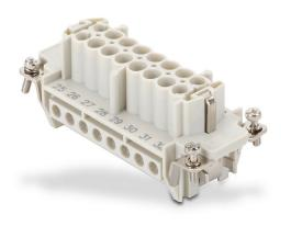
ZIPport female insert, connector housing size 16B, 16-pole, screw terminals, accepts wire size 20-14 AWG, 16 amp, 600 VAC/VDC, poles numbered 17 to 32. For use with ZIPport multi-wire housings.
