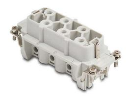
ZIPport female insert, connector housing size 16B, 6-pole, screw terminals, accepts wire size 20 - 10 AWG, 35 amp, 600 VAC/VDC, poles numbered 1 to 6. For use with ZIPport multi-wire housings.
