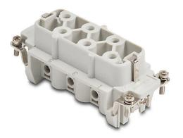
ZIPport female insert, connector housing size 16B, 6-pole, screw terminals, accepts wire size 20-10 AWG, 35 amp, 600 VAC/VDC, poles numbered 1 to 6. For use with ZIPport multi-wire housings.
