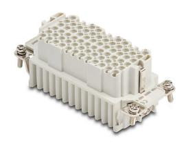
ZIPport female insert, connector housing size 16B, 72-pole, crimped contact, 10 amp, 600 VAC/VDC, poles numbered 1 to 72. For use with ZIPport multi-wire housings. Requires 10 amp female contacts ZP-MC-CC-F10A-xxx.
