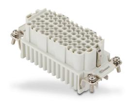
ZIPport female insert, connector housing size 16B, 72-pole, crimped contact, 10 amp, 600 VAC/VDC, poles numbered 73 to 144. For use with ZIPport multi-wire housings. Requires 10 amp female contacts ZP-MC-CC-F10A-xxx.
