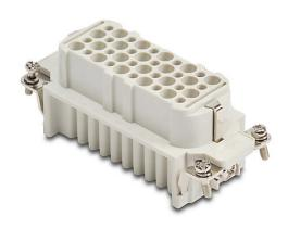
ZIPport female insert, connector housing size 16B, 40-pole, crimped contact, 10 amp, 600 VAC/VDC, poles numbered 1 to 40. For use with ZIPport multi-wire housings. Requires 10 amp female contacts ZP-MC-CC-F10A-xxx.
