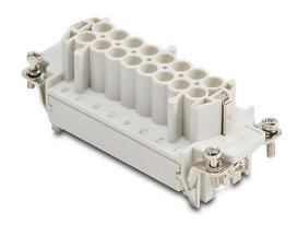
ZIPport female insert, connector housing size 16B, 16-pole, crimped contact, 16 amp, 600 VAC/VDC, poles numbered 1 to 16. For use with ZIPport multi-wire housings. Requires 16 amp female contacts ZP-MC-CC-F16A-xxx.
