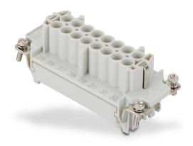
ZIPport female insert, connector housing size 16B, 16-pole, crimped contact, 16 amp, 600 VAC/VDC, poles numbered 17 to 32. For use with ZIPport multi-wire housings. Requires 16 amp female contacts ZP-MC-CC-F16A-xxx.
