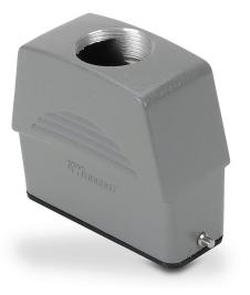
ZIPport hood housing, 2-peg, top entry, connector housing size 16A, (1) Pg 21 threaded hole, high construction, heavy-duty die cast aluminum. For use with ZIPport size 16A single lever connector housings.
