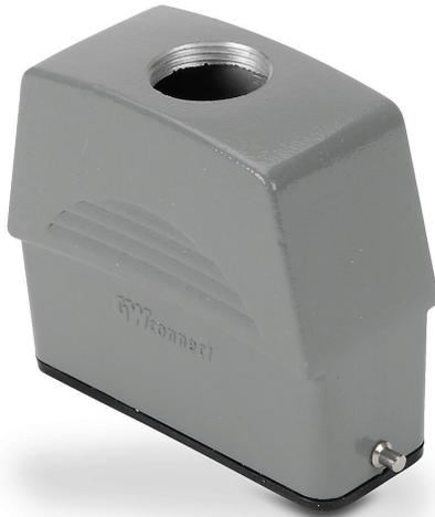
ZIPport hood housing, 2-peg, top entry, connector housing size 16A, (1) Pg 16 threaded hole, high construction, heavy-duty die cast aluminum. For use with ZIPport size 16A single lever connector housings.
