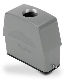
ZIPport hood housing, 2-peg, top entry, connector housing size 16A, (1) Pg 16 threaded hole, high construction, heavy-duty die cast aluminum. For use with ZIPport size 16A single lever connector housings.
