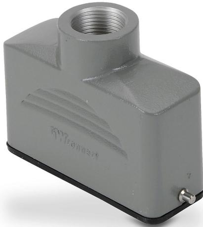
ZIPport hood housing, 2-peg, top entry, connector housing size 16A, (1) Pg 13.5 threaded hole, heavy-duty die cast aluminum. For use with ZIPport size 16A single lever connector housings.
