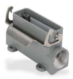
ZIPport surface mount housing, single lever, connector housing size 16A, (2) Pg 21 threaded holes, heavy-duty die cast aluminum. For use with ZIPport size 16A 2-peg connector housings.
