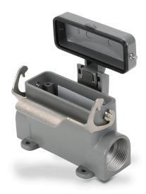
ZIPport surface mount housing, single lever, standard, connector housing size 16A, (2) Pg 21 threaded holes, heavy-duty die cast aluminum. For use with ZIPport size 16A 2-peg connector housings.
